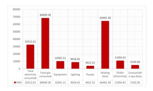
Figure 5. Amount of energy consumed by sections in 4 residential units using fan coils.
