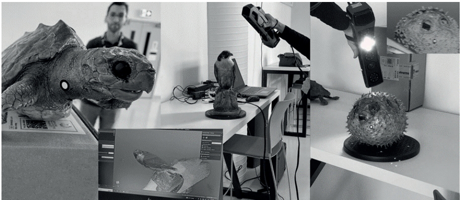
(Left to right) Turtle with a marker to aid reconstruction; live 3D reconstruction of peregrine (center); and porcupine fish (right).
