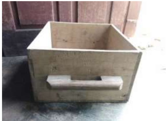
Figure 6. The measuring tool tông is made from wood (photo by Dini Hanifa)
