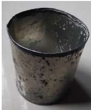
Figure 15. The measuring tool plôk ni is made from condensed milk cans (photo by Dini Hanifa)
