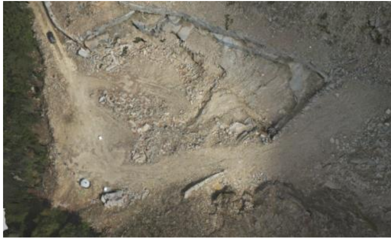
Fig. 8 - The orthophotos mosaic obtained after the triangulation.
