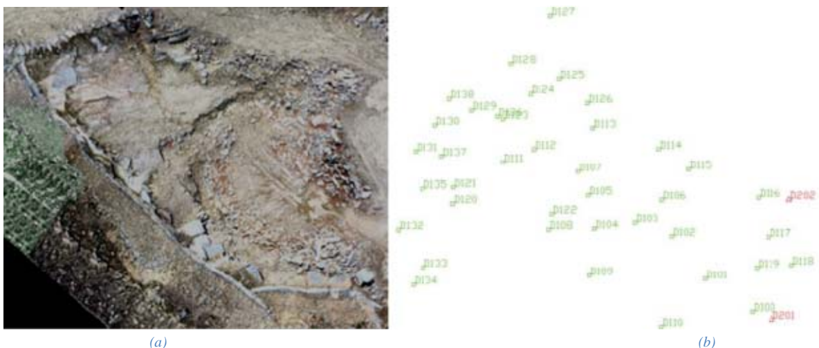
Fig. 2 - The GNSS vertexes (red) and the surveyed points (green).
