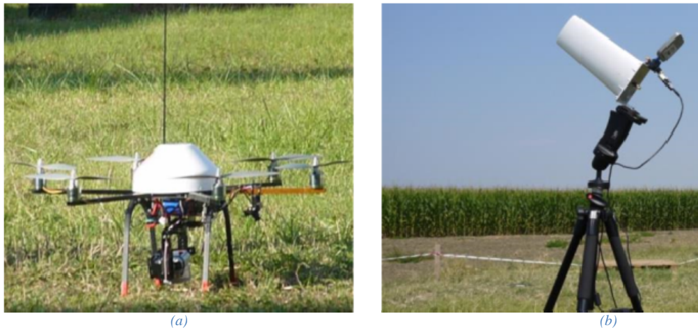
Fig. 3 - The UAV (a) and the antenna used for the telemetry.
