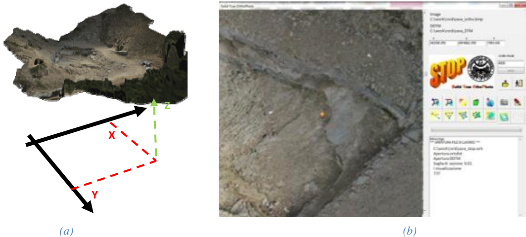
Fig. 10 - The Solid OrthoPhoto generated (a) and an example of STOP viewer (b).
