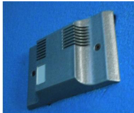
Fig. 3 - Temperature sensor mounted on wall bedroom.
