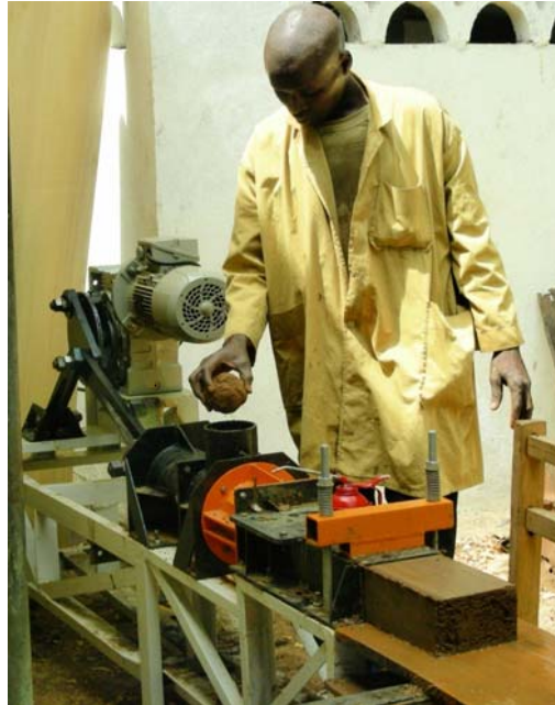
Fig. 6 - Earthen brick machine constructed in Cameroon.
