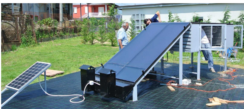
Icaro solar dryer under final preparations for testing
