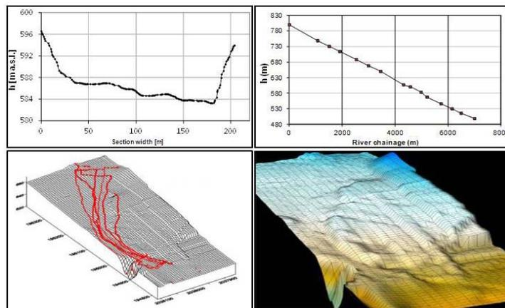
**Fig. 6** - Results of the topographical survey: example of a river cross-section (up-left; see also traces on Figure 1), longitudinal profile of the upper part of the River Soliette (up-right), post-processed analysis with survey tracks and digital elevation representation of surveyed area (bottom panels).
