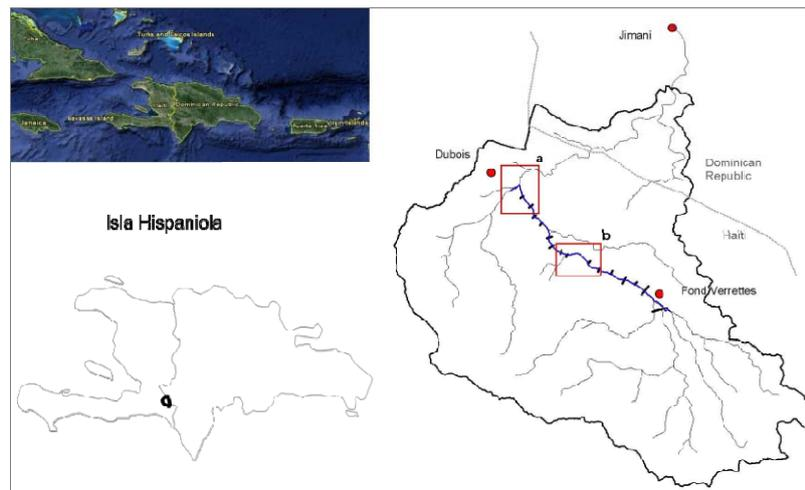
**Fig. 1** - Trans-boundary catchment of the River Soliette: principal hydrograph network (black tin line), modeled reach (blue tick line) and river cross-sections (black segments); red boxes identify the areas of interest for detailed topographic surveys.
