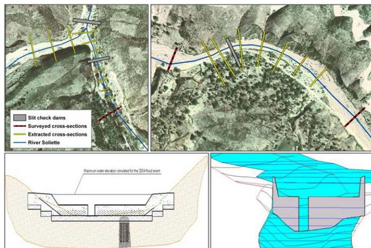
**Fig. 7** - Position of designed check-dams for boxes a (upper left panel) and b (upper right panel) of Figure 1; bottom left: frontal view of a slit dam characterized by the vertical opening of about 5 m width; bottom right: three-dimensional view of the River Soliette as implemented in the 1-D hydraulic model.
