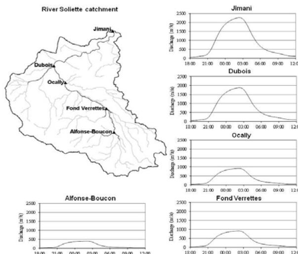
**Fig. 4** - Sections of interest of the Soliette catchment with relative flow hydrographs reconstructed for the May 2004 event by means of a quasi-distributed hydrological model (see [2] for more details).
