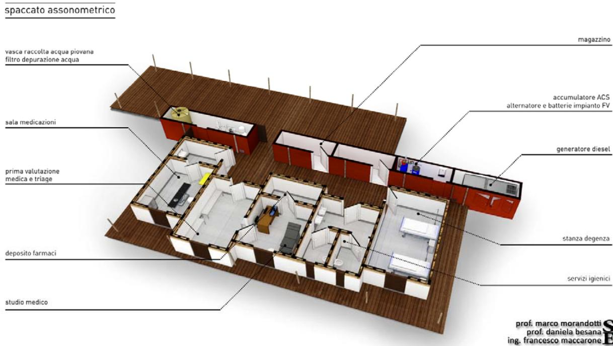
Fig. 5 - Functional layout of the dispensary unit.
