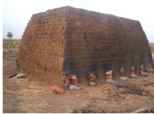
**Fig. 4** - Typical stove brick kiln.
