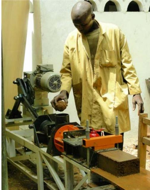
Fig. 6 - Earthen brick machine constructed in Cameroon.
