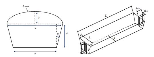
Fig. 2- Tubular section and trench geometries
