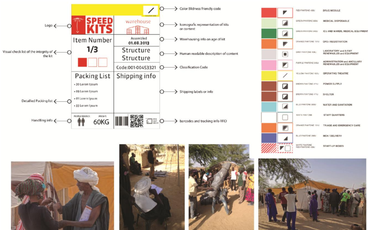
Image 5 – The packaging guidelines provided mounting instructions and tracking system; they were labeled with different colors according to the kit type. The photos show the field mounting test of the T1 – Clever Roof and T3 – Cocoon, in Senegal.
