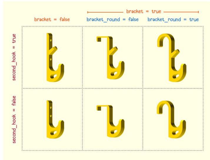
Figure 10: Different U-Hook designs with matching parameters (Payen, 2016).
