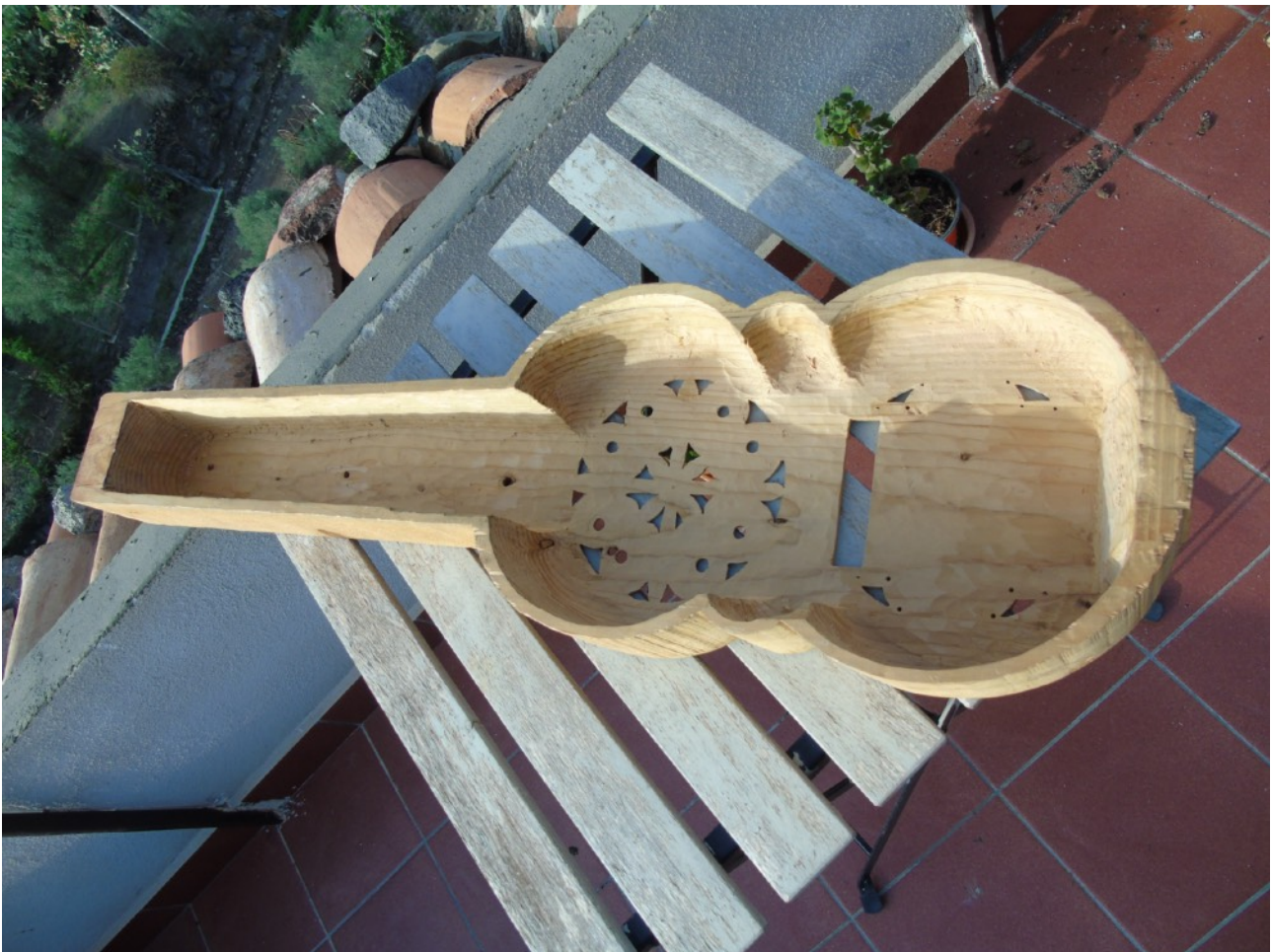
Figura 11: Carving the soundbox in a cedar trunk.
