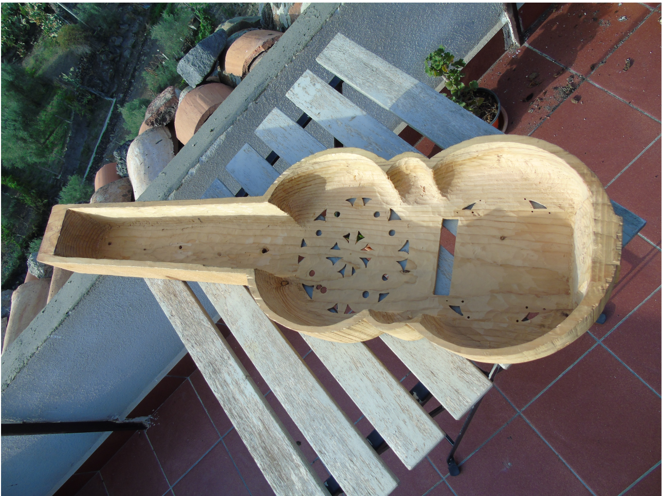
Figura 11: Carving the soundbox in a cedar trunk.
